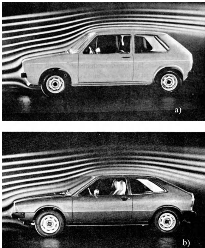
FIGURE 21.7. Streamlines in the symmetry plane about two fastback cars. In (a) the flow detaches at the end of the roof while in (b) it remains attached up to the end of the trunk.
